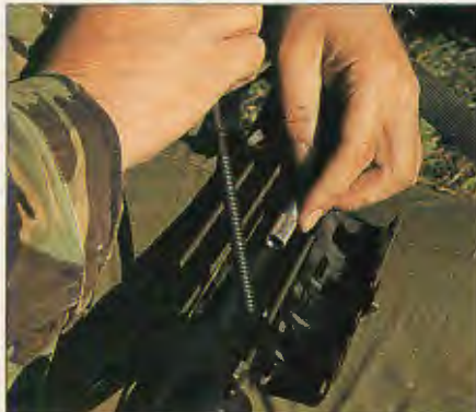
8 Pull out the piston and its spring. The spring stays on the piston, and should not be removed. Take out the gas plug by depressing and pushing it through its housing.
